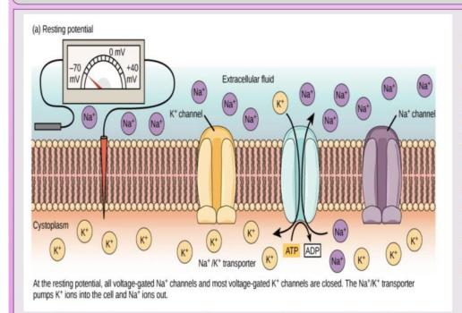
Voltage-gated channels can open or close and allow a surge Sodium and Potassium ions to pass through. Voltage and current in the system are caused by charged ions moving the across membrane.
